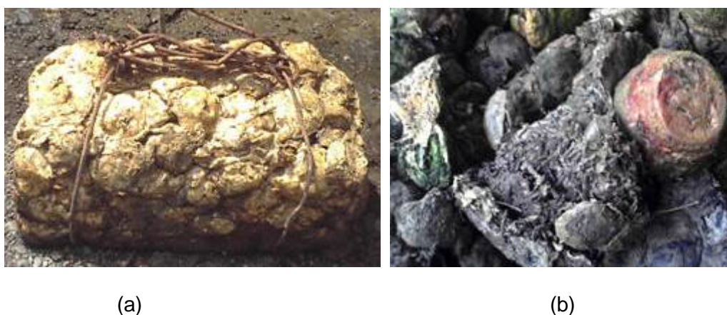
Figure 5. Raw rubber material produces by farmer. A quite clean cup lump (a) and dirty cup lump (b)
